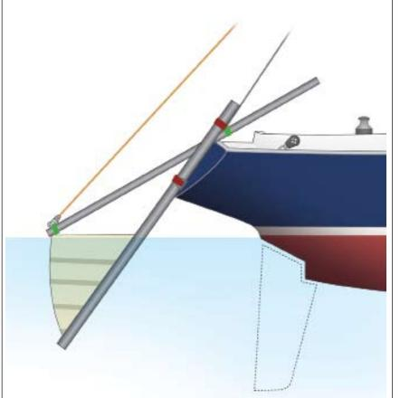
Essentially a sail on a pair of spars, the "soft rudder" was developed by U.S. West Coast naval architect Paul Kamen. Visit www.well.com/~pk/PCrudder-04. htm for more information on his emergency-steering solutions.
