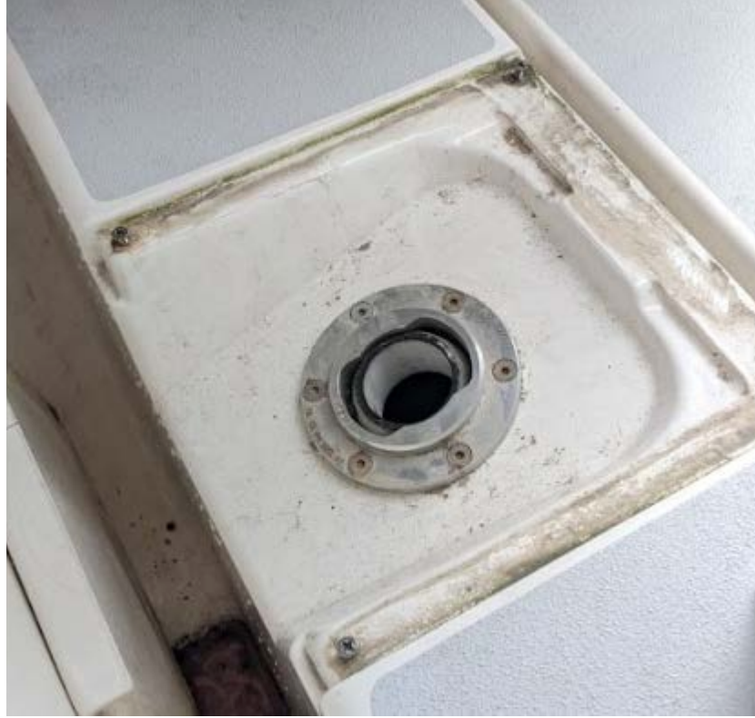
Figure 4 The upper rudder bearing aboard Alliance when viewed from on deck. Note that the bearing is located immediately aft of the wheel well (visible) in the cockpit sole and is normally covered by a removable fiberglass plate.
