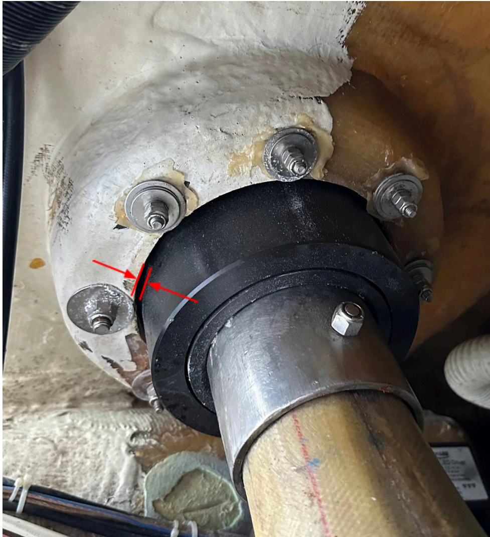
Figure 5 A loose-fitted upper rudder bearing (vessel type not specified). Note the gap between the external face of the bearing and the structure in which it is mounted. In this case, all lateral loads are dependent on the through-bolted fasteners.
