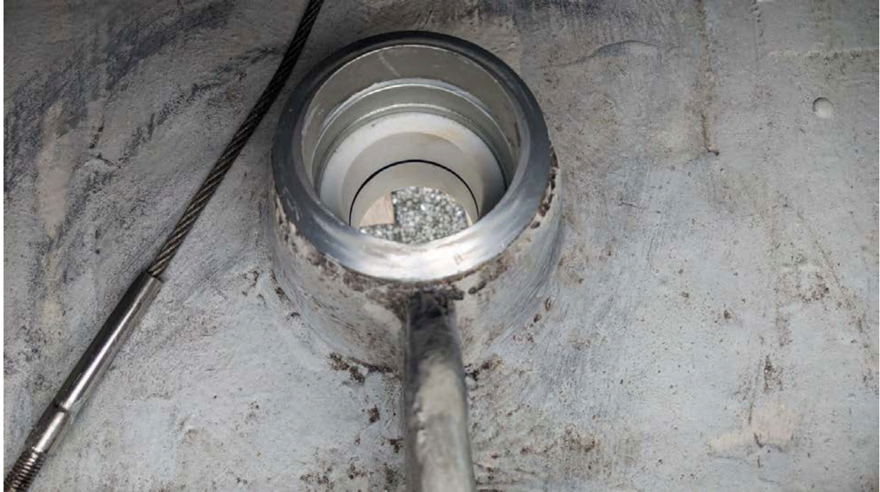
Figure 3 A photograph of the lower bearing on Alliance and its fiberglass and aluminum housing. This picture is taken from aft looking forward. Note the longitudinal support immediately aft of the structure.
