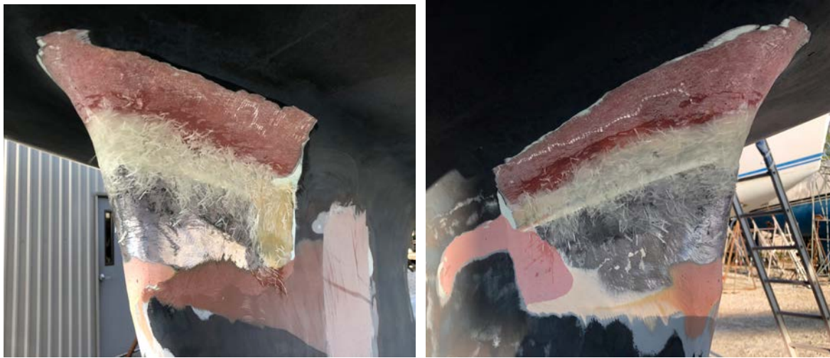
FIGURE 9 – Photos of repairs to the hull – keel interface taken during November, 2023 repairs to the keel.
