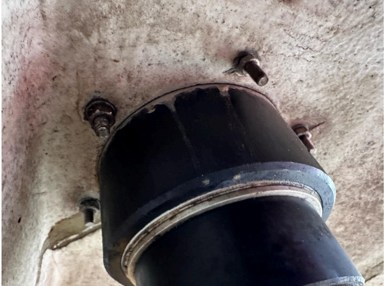
Figure 6 Photo supplied by PYI, Inc., of a properly fitted upper rudder bearing (vessel type not specified). Note the tight tolerance between the outside of the bearing and the surrounding deck structure.
